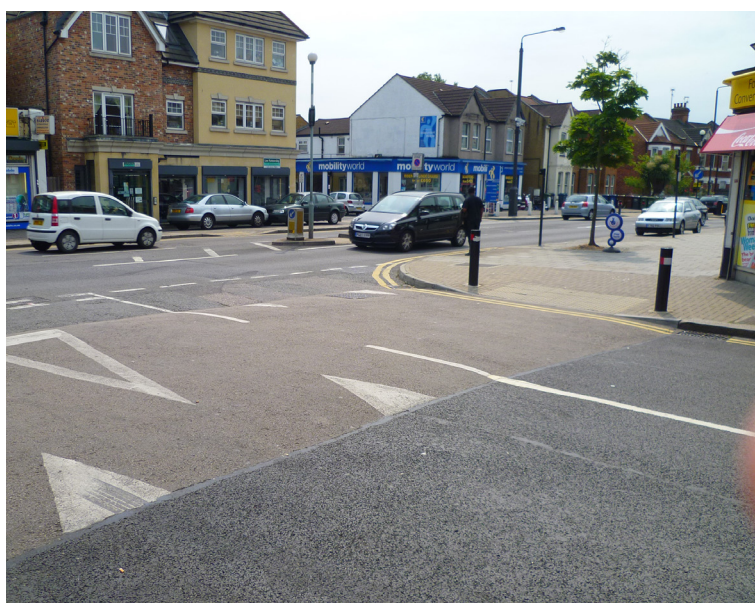
Typical Raised Entry Treatment
